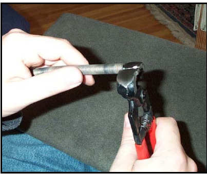
Figure 20. Cutting individual rings w/ overlap
