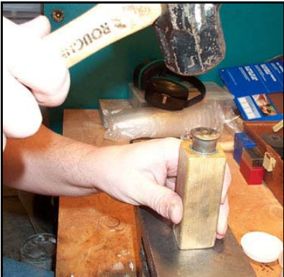
Figure 21. Flattening rings with piston tool
