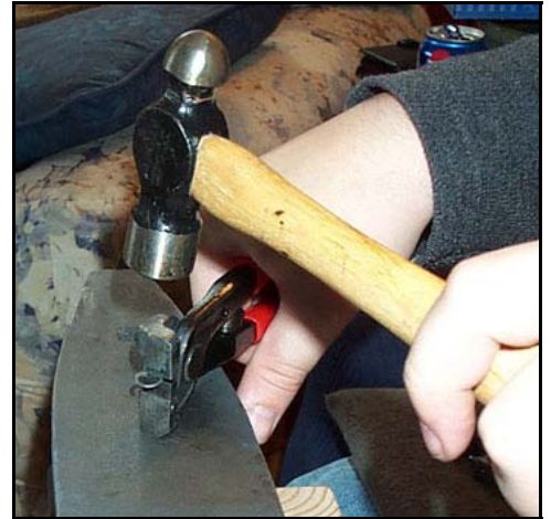
Figure 23. Setting wedge rivet
