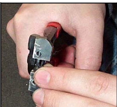
Figure 22. Piercing hole for wedge rivet
