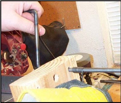
Figure 19. Winding coils on mandrel
