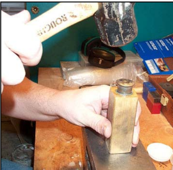
Figure 18. Flattening rings with piston tool
