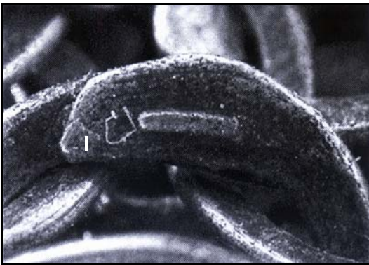
Figure 10. Wedge rivet back, Wallace collection A9 15th c. (Schmid, p. 13)
