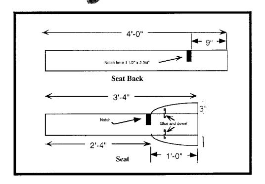
Materials required: 10 linear feet of 2 x 6 lumber, carpenters' wood glue, 3/8" dowels
